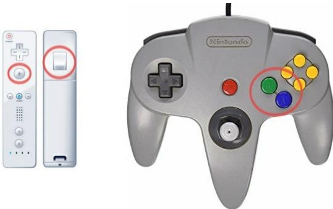
Image 4.3: Comparison of A and B button placements between Wii Remote and N64 controller.
